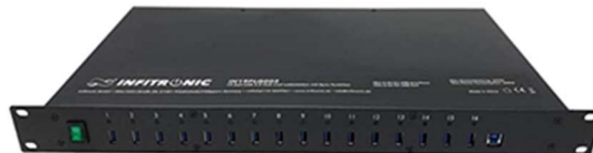
Figure 29. USB HUB with 16 ports installed initially.
